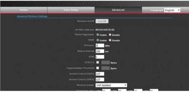
Within the "Wireless On / Off" option you can use the "Turn On / Off" button to turn on/off your wireless network. Below it shows the MAC address of the access point. Furthermore, it is possible to turn on/off the "Packet Aggregate" and the "WMM".
