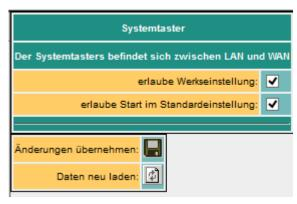
allow factory settings 🗹 The device can be set to the delivery condition
