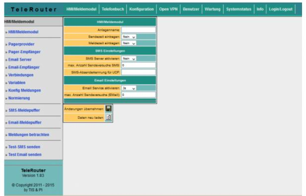
With the HMI message module, SMS and email messages (fault messages and maintenance messages) can be sent automatically to virtually any number of recipients, depending on the event, in the PLC, without any programming effort. The system automatically assigns the messages to the respective recipients and sends the message via the correct provider.
