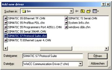
7. In the dialog "Add new driver" select the driver which fits to your PLC For a S5 PLC, you can choose the file SIMATIC S5 Programmers Port AS511.chn. If you are using a different PLC please inform yourself which driver fits with your PLC.
