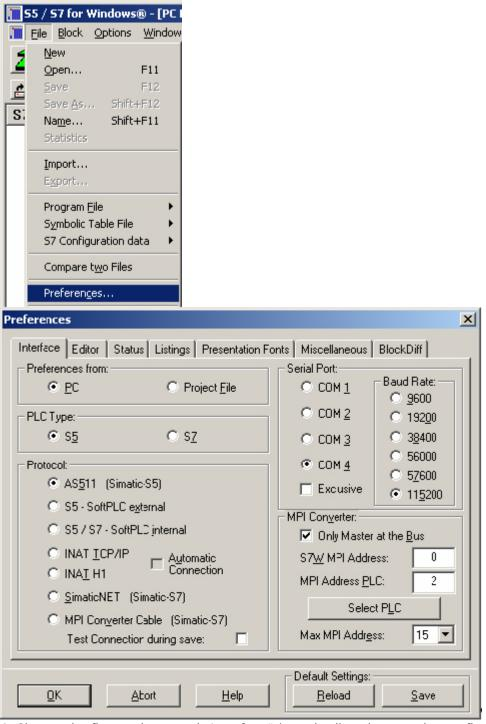
4. Choose the first registry card "Interface" (standard) and set up the configuration data as descriped below:  $\Rightarrow$  Interface Settings from : "PC"
