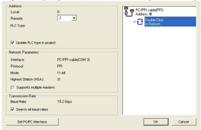
3. Click on "Communications…" to start the next dialog. In the sector "Address" set up the "Remote" listbox with the station address of the PLC (e.g. "2").
