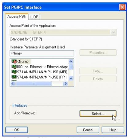
3. A Dialog with a list box named "Interface Parameter Assignment Used:" appears. This box should offer some "PC - Adapter" entries If this is the case, please continue with the step MPI settings or Profibus settings. If you can't find these entries go ahead with step PC-Adapter or TCP/IP installation.
