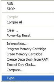
Select a CPU type and version, or read the PLC type from the PLC if you would like the software to range-check parameters for the PLC's allowable memory ranges.
