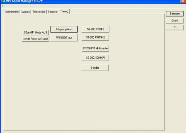
This tab is only used in some special cases. If you press the button "Check Adapter" the cable is connected und after that the following dialog is displayed:
