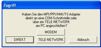
For access query choose "Direct" if your product connects via USB-cable or Nullmodem-cable. "Modem" if your product connects via telephone line or "TELE-Network" if your product connects with a TELE-Network device via telephone line. The bars below shows at which COM-port something was found or not.
