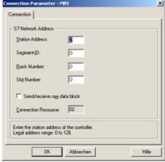
9. Now you are able to type in the name of the connection. With a click on "Configuration" a new dialog will appear. Now you are able to set the properties of the connection. Set up the station address of the PLC (in this example "2"). Confirm with "OK" until you are back to the main window. Read further "Communication and fault diagnosis ".
