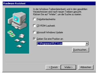
13. Activate the checkbox "Set the driver position:" and deactivate all the others. Click on "Choose..." and choose the path where the PLC – VCom software is installed. Confirm your configuration with "OK" and click on "Next".
