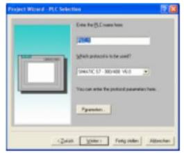
4. "Next" leads you to a new dialog. Type in the specific fields the name of the PLC device and choose the used PLC in the driver selection (e.g. "SIMATIC S7 – 300/400 V6.0").
