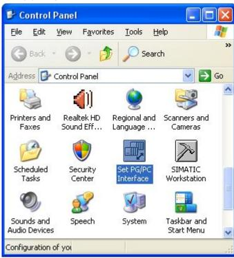
1. Open the system configuration by using the start menu. 2. Click on "Set PG/PC interface".
