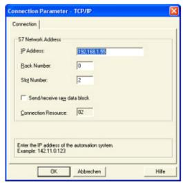
10. A dialog appears where you can configure the connection parameters. Set up the IP - Address of the module and configure the rack number as well as the slot number. Confirm this configuration by clicking "OK". Example configuration:
