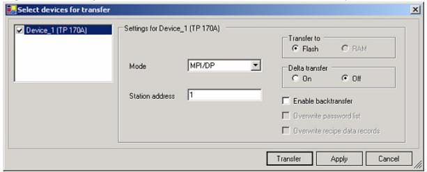
9. Press the button "Transfer" to start communication with the terminal. Your project is about to be transferred. The WinCC flexible software is now able to communicate with your operator panel.
