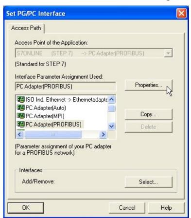
24. If you want to use ProTool/Pro RunTime you can set the "PG/PC Interface" by selecting the entry "DPSONLINE". Therefore you have to select "Access Point of Application" and configure it as described above. The easiest way is to use the S7-LAN/MPI-LAN/MPI-USB- driver which supports USB and LAN products.
