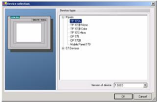
3. In the "Device selection" mark the used operator panel (example: "TP 170A") confirm with "OK".
