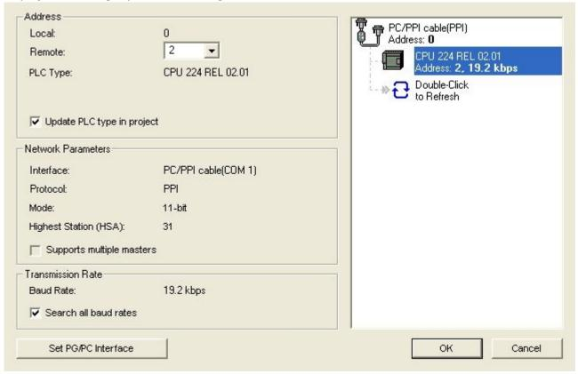
6. Confirm with "OK" until you get back to the main window. The communication with the PLC ist now established.
