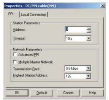
9. In the menu "Local Connection" you select the com-port "Interface to" to the port which is served from the tool PLCVCom. 10. Click on the button "OK" and click in the left down area in your windows on "Communikations".
