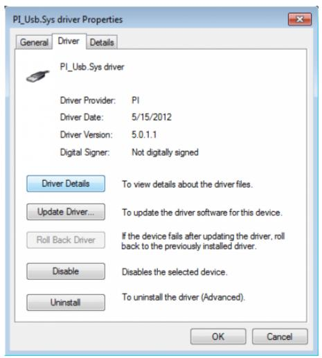
If the driver has to be deleted, please use the function "Uninstall" and set the check-box in "Delete the driver software for this device":
