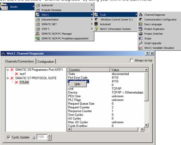
20. The tool could not detect a running connection so it marked the connection/s with a red 'X' (registry card "Channels/Connections"). Click on the last created, not active connection (with the red 'X') and some informations from the connection will appear in the right part of the dialog. One of these counters is called "Last Error Code".
