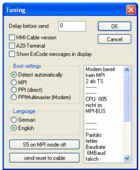
The following configuration is possible, it will be transferred to the Cable by pressing the button "OK". The configuration is saved permanently in the Flash-ROM:
