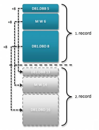
The chart shows what and how much is read when the option **Number of records** is set to the value **two** and also the option **data byte offset** is set to the value **8**.
